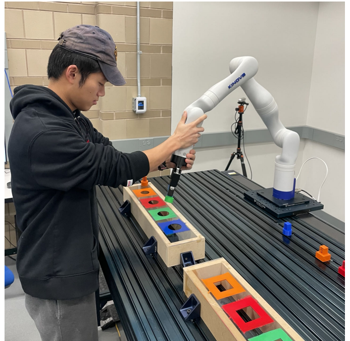
Figure 1: A human providing kinesthetic feedback to a robot arm while it is performing pick-and-place tasks.
