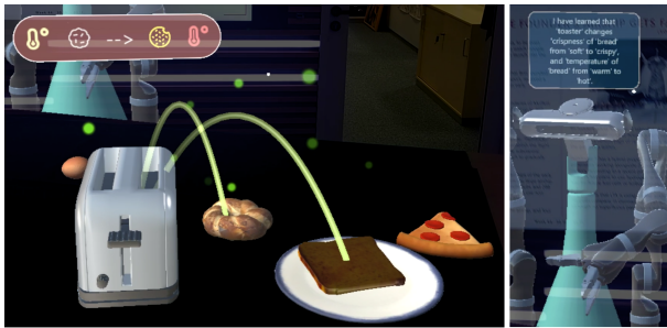
Figure 3: Graphical elements used to explain to the user that the robot learned that food items in the "bread" category can be heated up in the toaster (left). The same message is also provided by text (right) and speech.
