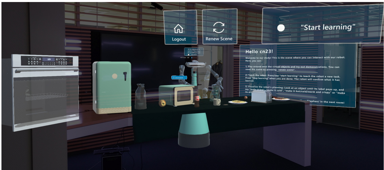
Figure 1: The AR scenario for the robot training and interaction with the user. The scene is a common office space with a table upon which holographic kitchen items are displayed. Virtual controls (to log out, reinitialize the scene, and initiate a teaching episode) were displayed on the upper visual field of the person wearing AR glasses and moving rigidly with the user's head.
