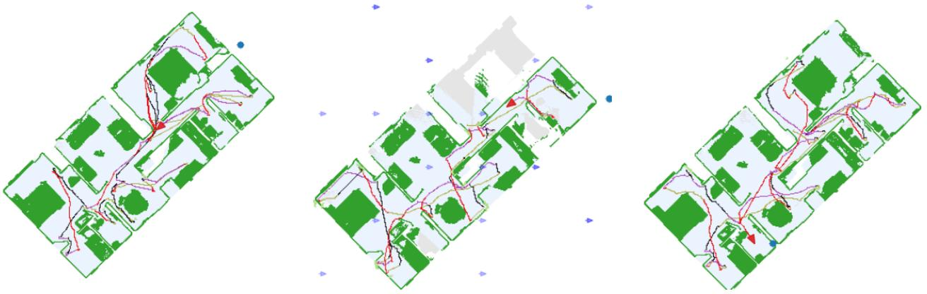
Fig. 2. Original mapping and navigation (**Left** 88 ops) under right-side influence (**Middle** 24 ops). **Right**: Resulting influenced policy. The trajectory of the SLAM agent is indicated and the color indicates the orientation of the agent while traveling. Red is south, Black is north, Pale green is east, and purple is west oriented.
